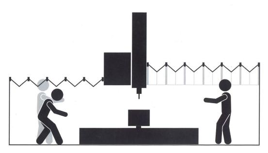
even machines with a reduced Z-axis, while allowing the machine operator to access the machining chamber without opening the cover. Wave Cover is based on a modular system similar to Wave Sky. The shape, however, resembles more that of a gable roof, which provides for more headway and allows positioning the cover at every height of the guideways".
