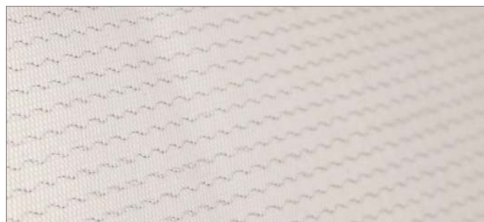
Detail of the antistatic feature of the fabric
