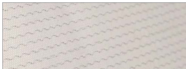
Detail of the antistatic feature of the fabric
